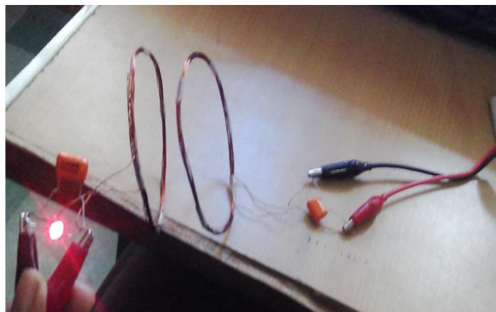
Fig. 10(a) Experimental setup showing parallel coupled resonators with LED as load.
